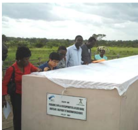
Sun drying system (concrete with dust protector).
